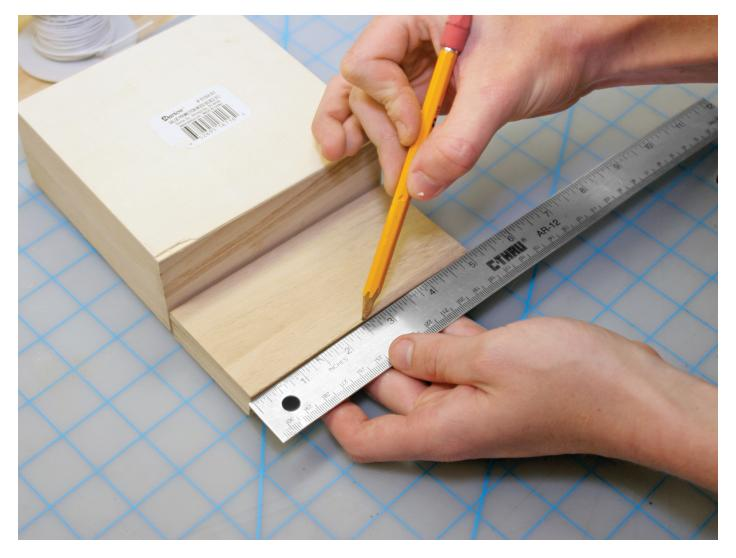
Mark the positions on the templates where they meet: the toggle and bracket's position on the lid, and the motor and switch's position on the bracket.
